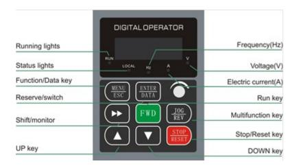
Fig. 4-3 Control panel diagram
