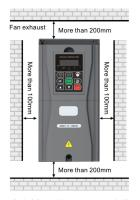
Figure 3-1 Mounting space and distance
